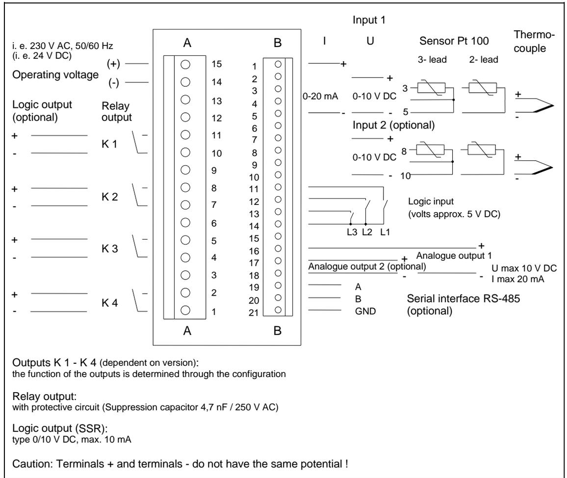
**1.3 Terminal connection diagram DPG 96 C / DPP 96 C (depending on version)**
